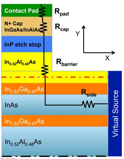
Contact resistance between the channel and the contact pad.
