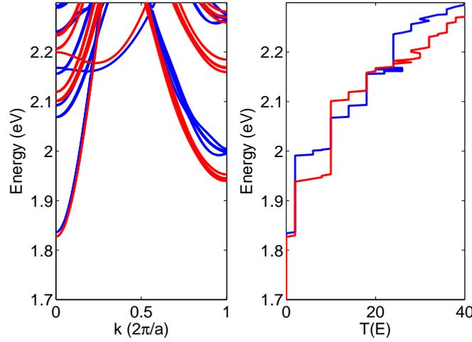
**Figure 3.** Comparison of E-k diagram of conduction bands (left figure) and Transmission (right figure) of GaAs nanowire . The red lines are results using TB parameters generated by this work; the blue line are results using TB parameters by ref[9].
