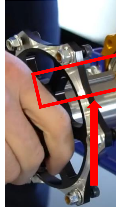
Key under sprocket hub
