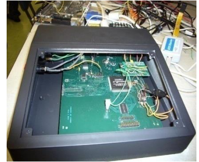
Final Printed Circuit Board (PCB)
