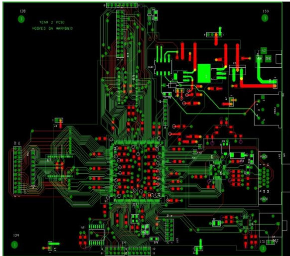
4-layer Printed Circuit Board (PCB)
