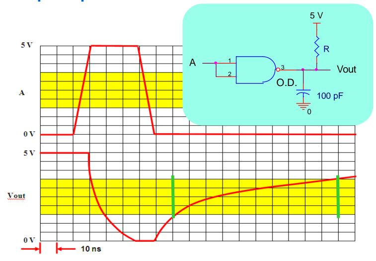
rise time = 100 ns =  $R_{pull-up}$  x 100 pF  $\rightarrow$   $R_{pull-up}$  = 1000  $\Omega$
