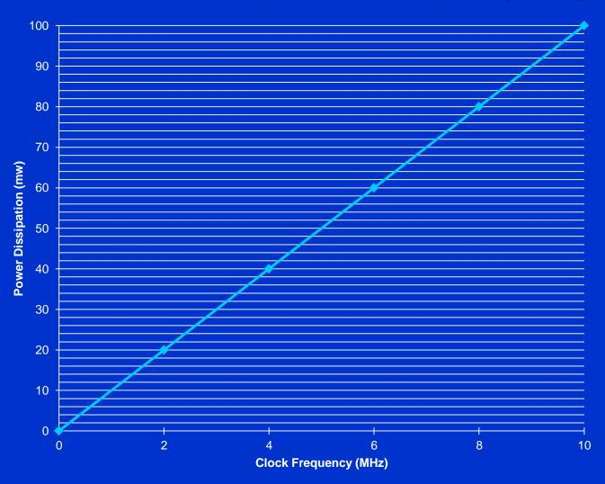
Example - A microcontroller can operate over a power supply range of 1 to 5 volts, and dissipates 100 mW when operated at 5 VDC; plot its power dissipation over the specified power supply range
