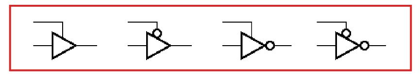
Basic variations: The buffer may be inverting or non-inverting, and the tri-state enable can either be active low or active high
