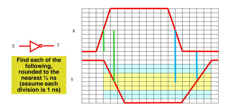
Rise propagation delay  $(t_{PLH}) = 3$  ns
