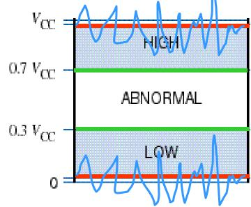
DC noise margin is a measure of how much noise it takes to *corrupt* a worst-case output voltage into a value that may not be recognized properly by an input
