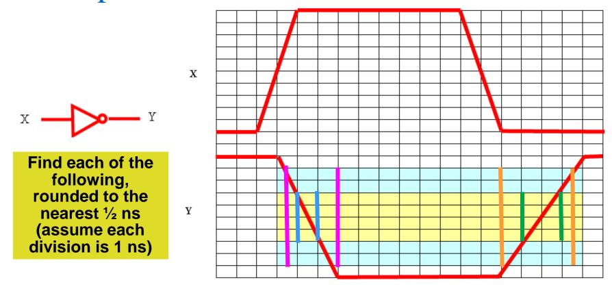
Rise time ( $t_{TLH}$ ) based on Wakerly's (30%-70%) definition = 2 ns Rise time ( $t_{TLH}$ ) based on standard 10%-90% definition = 3.5 ns Fall time ( $t_{THL}$ ) based on Wakerly's (70%-30%) definition = 1 ns Fall time ( $t_{THL}$ ) based on standard 90%-10% definition = 2.5 ns
