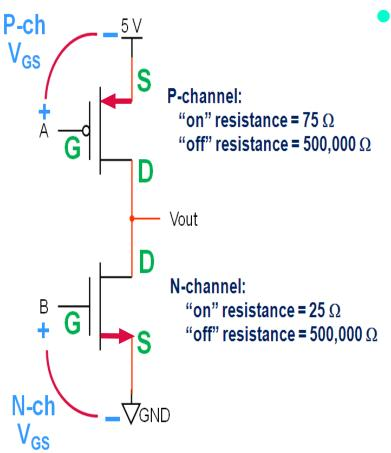
Calculate V<sub>out</sub> for the case A=5V, B=0
