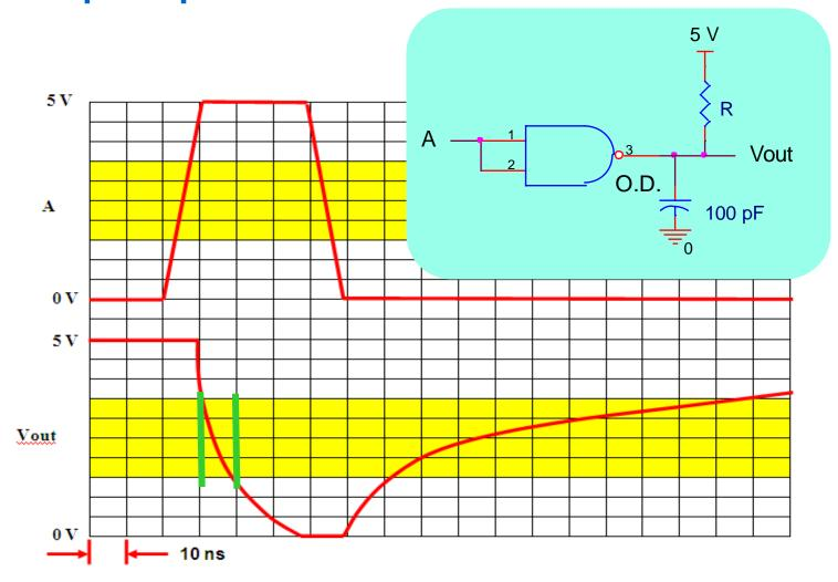
fall time = 10 ns =  $R_{on}$  x 100 pF  $\rightarrow R_{on}$  = 100 $\Omega$
