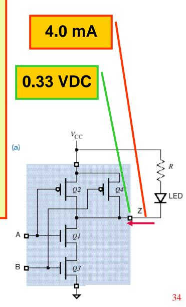
**Example:** Based on the data provided in Table 3-3 of the course text, calculate the value of the LED current limiting resistor for the <u>worst case</u> *current sourcing* configuration. Also calculate the amount of power dissipated by the current limiting resistor. Assume  $V_{LED}$  is 1.9 volts.
