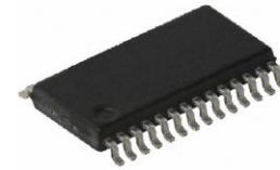
Shrink Small-Outline Package (SSOP)
