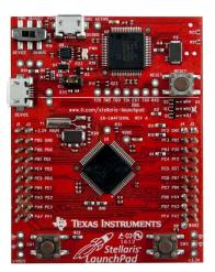
Using the included USB cable, connect the USB emulation connector on your evaluation board (marked DEBUG) to a free USB port on your PC. A PC's USB port is capable of sourcing up to 500 mA for each attached device, which is sufficient for the evaluation board. If connecting the board through a USB hub, it must be a powered hub.
