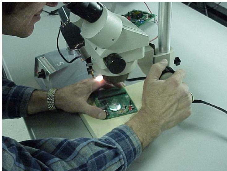
Figure 35. Stereo zoom inspection station (7X to 40X magnification) helps to inspect solder joint workmanship
