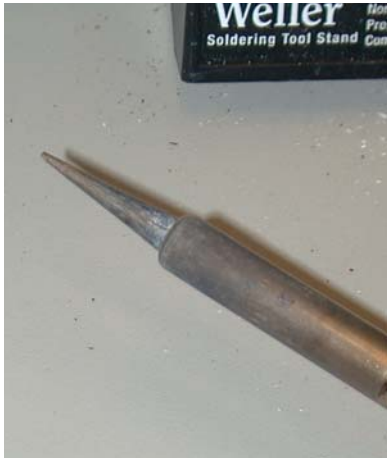
Figure 4. ESD safe soldering station with fine tip wand. This one is Weller model EC1201A
