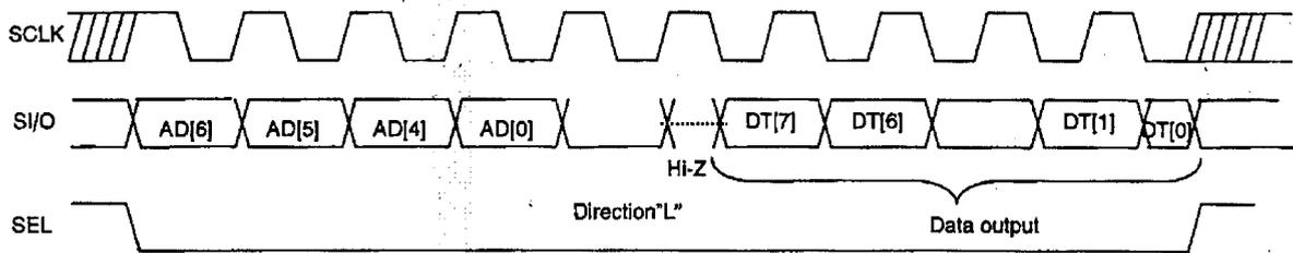
Read operation (SO output): Output is synchronized to a rising edge of SCLK.
