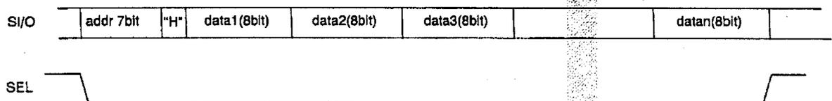
Read operation (S/O output): Output is synchronized to a falling edge of SCLK.
