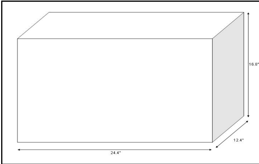
Fig 1.3: Prototype fish tank which will be used for project purposes (Front view).
