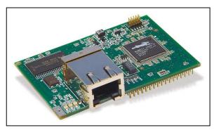
RCM3200 has 52 digital I/O pins; 44 configurable, 4 fixed input, and 4 fixed output. An internal battery backable RTC is extremely useful for our design as well.
