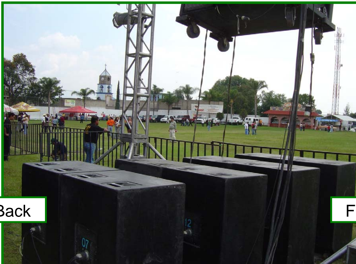
2 wide, 4 element end-fire array outdoors
