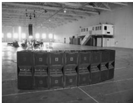
Fig. 44. Indoor ground-plane setup for vertical polar response measurements of eight-element curved array.
