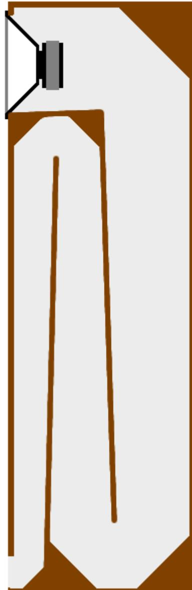
Length of transmission line has to be long enough to provide at least 90° of phase shift (1/4 of longest wavelength of interest)
