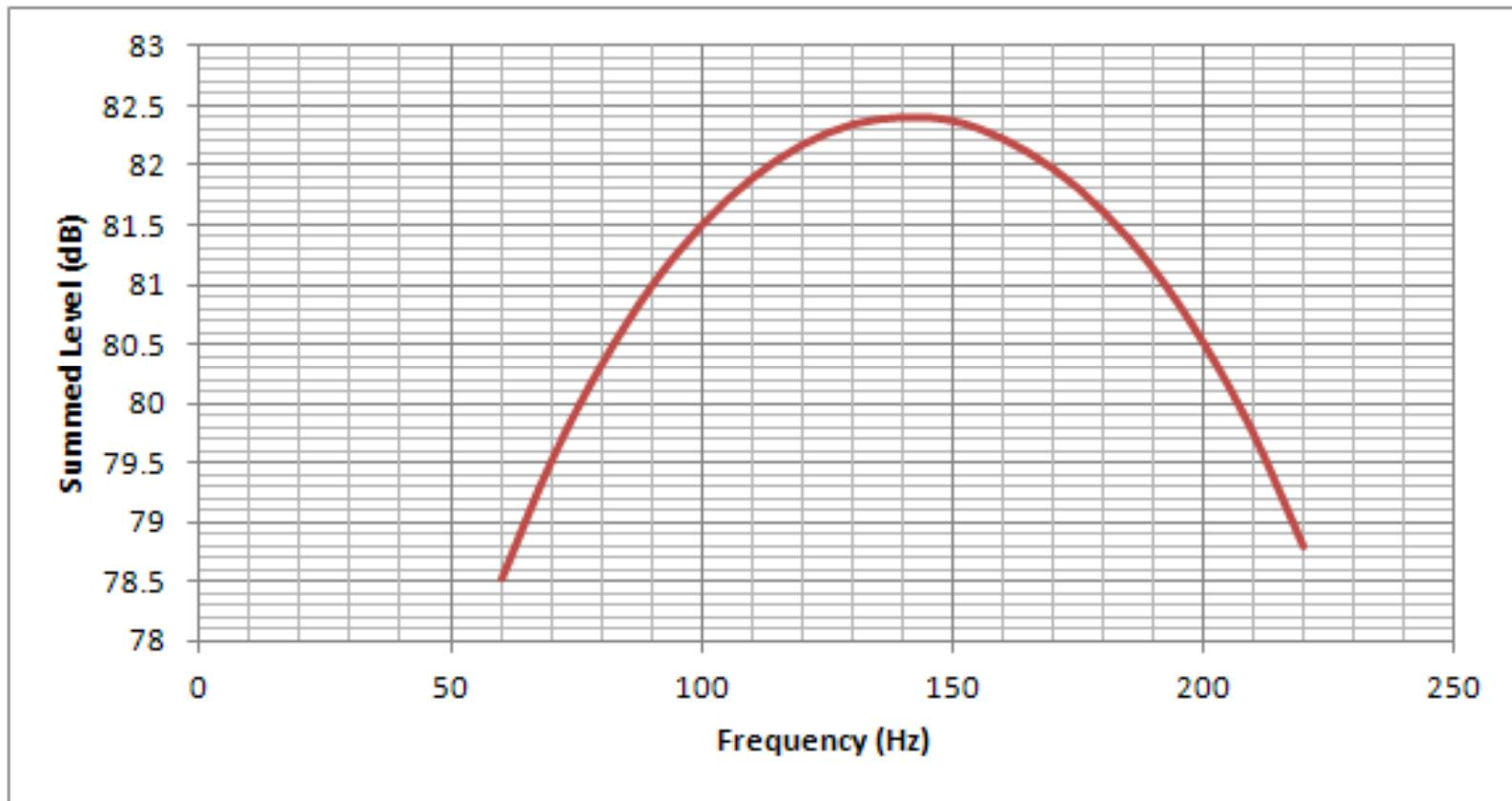
Problem: No way to “stop” (attenuate) rear radiation outside of this band (approx. 60 – 220 Hz) → leads to unacceptable amount of “combing”
