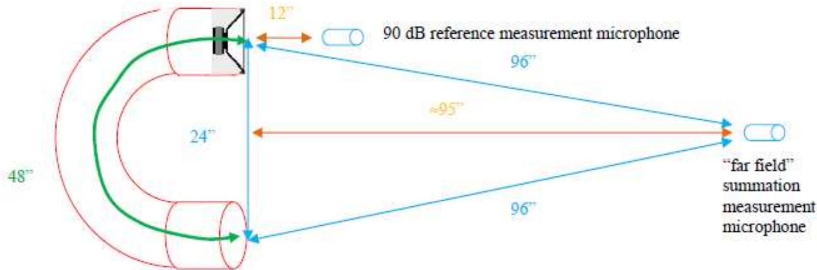
Determine the minimum frequency and the maximum frequency at which this undamped pipe should be allowed to operate (when observed in the “far field”, e.g. at a distance of approx. 95” on-axis with respect to the midpoint of the two openings, with the stuffing material and end cap removed). Also determine the frequency at which the summation peak occurs due to phase shift. In each case determine the dB SPL measured at the “far field” summation point.
