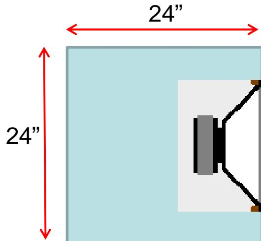
Don't forget: rear radiation is 180° out of phase with front radiation!
