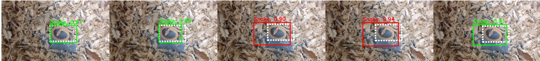
(b) Faster R-CNN + Multi-branch + our Content Aware Scheduler, or FR+MB+CAS chooses a branch of di = 50 , rd = 384 , nprop = 100 , rt = 25\% , and ct = 0.05 , given a 20 msec latency constraint.
