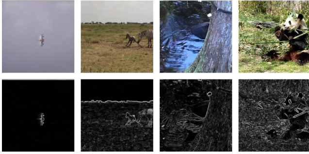
Figure 3.7. Sample frames (first row) and edge maps (second row), going from left to right as simple to complex. Normalized mean edge values from left to right: 0.03, 0.24, 0.50, and 0.99 with corresponding frame complexity categories: 1, 3, 6, and 7
