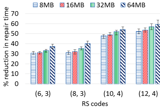
(a) Percentage reduction in repair time with PPR over baseline Reed-Solomon code for different chunk sizes and coding parameters
