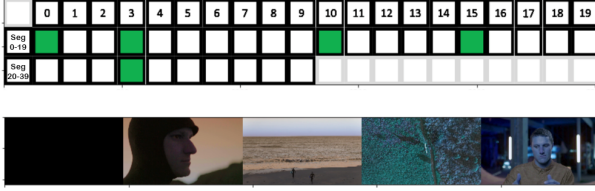
Fig. 2. Visualization of the Intermediate Representation for a video summarization application. A video shot is labelled in green if it is included in the summary, and in white otherwise. In this example, the summary includes five shots, namely 0th, 3rd, 10th, 15th, and 23rd shots. The first video frame of each shot is also shown.
