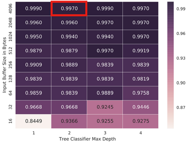
Fig. A2 – Recall Score on validation set for increasing buffer sizes and maximum depth of tree parameters. For our experimental evaluation, we select the parameters of tree depth of two and buffer size 4096 bytes. (For interpretation of the references to color in the discussion of this figure, the reader is referred to the web version of this article.)
