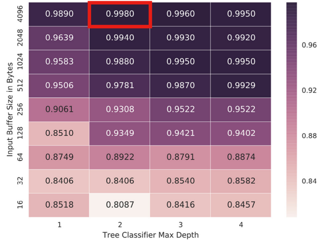
Fig. A3 – Precision Score on validation set for increasing buffer sizes and maximum depth of tree parameters. For our experimental evaluation, we select the parameters of tree depth of two and buffer size of 4096 bytes. (For interpretation of the references to color in the discussion of this figure, the reader is referred to the web version of this article.)
