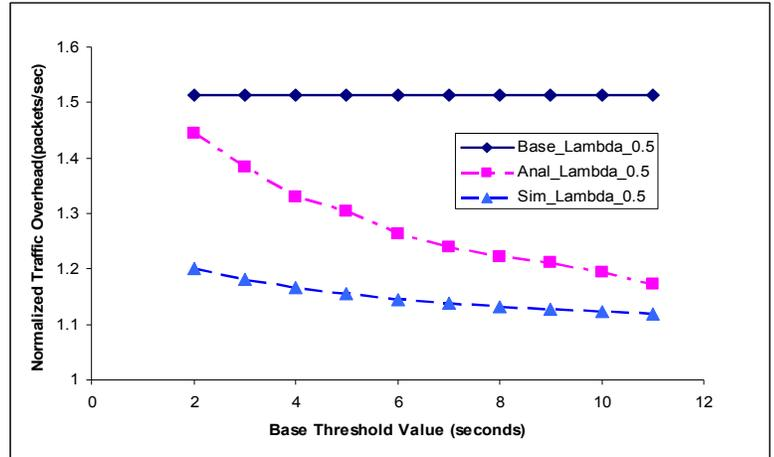
**Figure 2. Normalized traffic overhead due to SeNDORComm and GenericComm (Base)**
