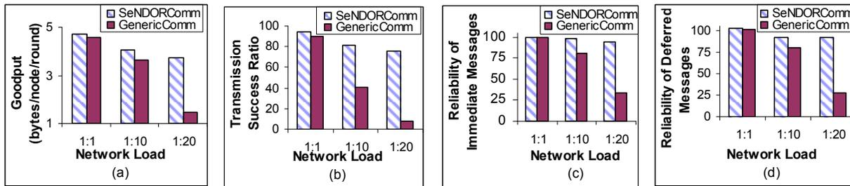
**Figure 5. Behavior of SeNDORComm and GenericComm under varying load conditions on a 100 node network simulation.**
