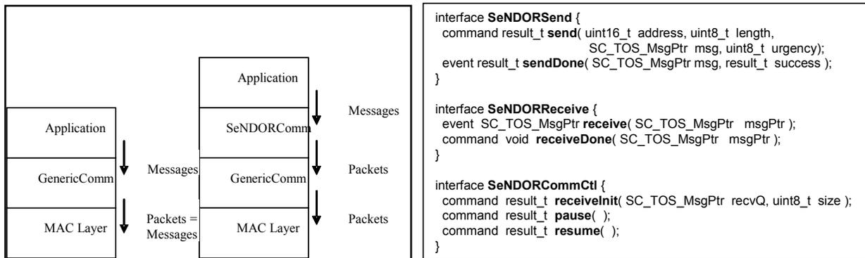
**Figure 1. WSN application's radio stack interface respectively without and with SeNDORComm(left). SeNDORComm Interfaces: Send, Receive, Control(right).**
