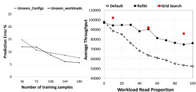
Performance of Cassandra with optimal configuration selected by Rafiki vs. default configuration. Three points are shown for the theoretically optimal performance using exhaustive searching.
