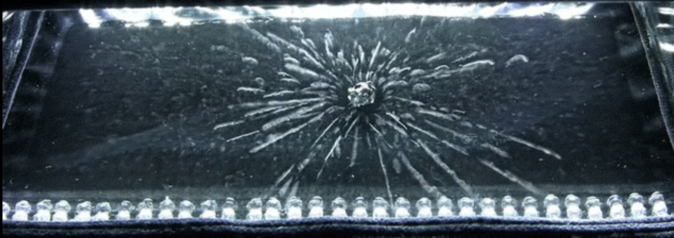
Uranium emitting radiation in a cloud chamber
