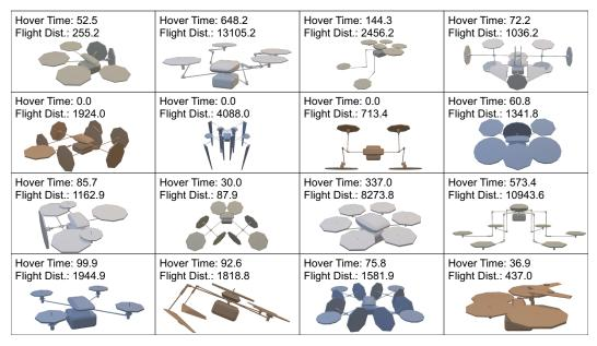
Figure 3: Diverse vehicle designs in AircraftVerse with different structures and with different performances. Some designs can hover in place. Hover time is in seconds and flight distance is in meters.
