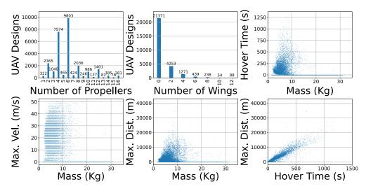
Figure 4: The designs in AircraftVerse exhibit diverse performance with respect to characteristics such as maximum flight distance and hover-time. They also have very different physical characteristics such as mass, number of propellers, and number of wings.
