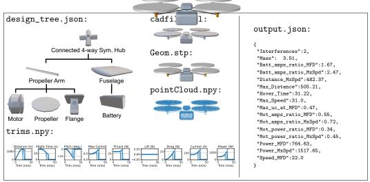
Figure 2: An illustration of all the key file components that make up an aircraft design. The design\_tree.json captures all aspects of the design (e.g. 4-way hub) that appears in both the cadfile.stl and the Geom.stp. Additional files of design\_seq.json and design\_low\_level.json are directly derived from the design tree. The performance of the aerial vehicle is displayed in both the performance file labeled output.json and in the trims.npy.
