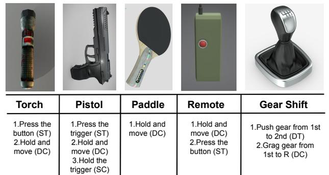
**Figure 17: User Study: 5 virtual objects covering 4 Interactions which Static Transient (ST), Static Continuous (SC), Dynamic Transient (DT), and Dynamic Continuous (DC)**
