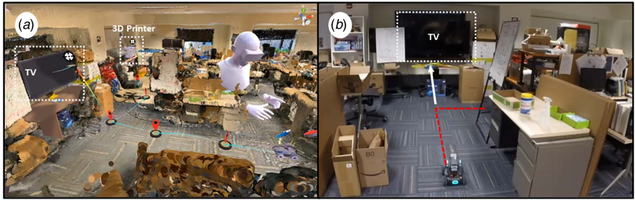
Fig. 15 Robot-IoT use case: (a) user specifies the path and authors actions in VR and (b) the physical robot performs the tasks as authored by human in real world
