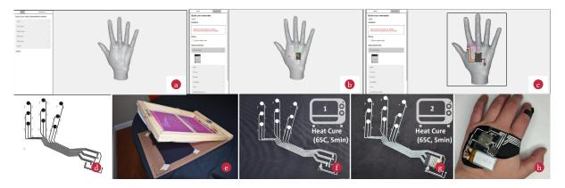
Fig. 5. Design and Fabrication Workflow: (a) Hand measurements parametrization, (b), Place desired components on the 3D handmodel, (c) Generate circuit wires (manually or autorouting), (d) generate and Print the template, (e) Screenprint circuits on nylon fabric using conductive silver ink, (f) heat cure the ink, (g) Assemble components on the circuit and heat cure the connections, (h) Hand wearing the prototype
