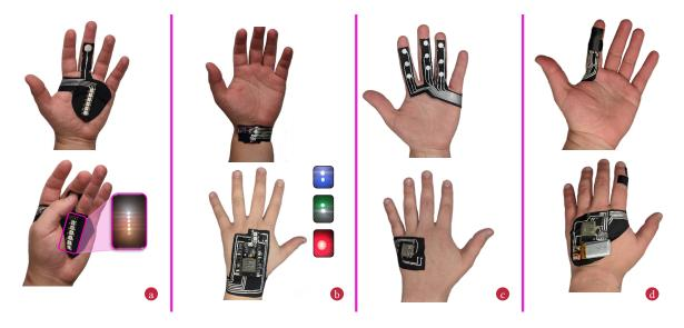
Fig. 7. (a) Hand Repulsor (9 components) (b) Pulse and Temperature sensor for constant monitoring (6 components), (c) Nine keys capacitive touch keyboard (11 components), (d) Piezoresistive touch input for Augmented and Virtual Reality (10 components)
