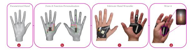
Fig. 1. A 3D parametric hand model (a) is interactively customized by adding electronic components (b) by using FabHandWear and then fabricated (c). The printed wearable device has the desired shape and function (d) .
