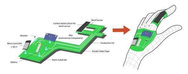
Fig. 6. FabHandWear System characteristics
