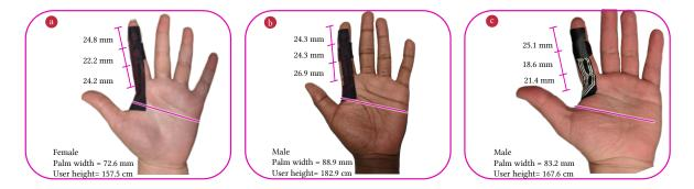
Fig. 8. Users fitting results of one of the hand wearable customization patterns. Illustration of the differences of hand features across users with a fitted design.
