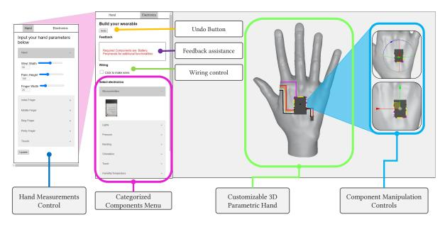
Fig. 2. FabHandWear Design Interface - Sections Description
