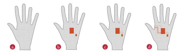
Fig. 4. The hand model is discretized with a 2D grid (a). After the circuits are positioned (b) the tool automatically finds routing connection of the components (c) and sensors (d).
