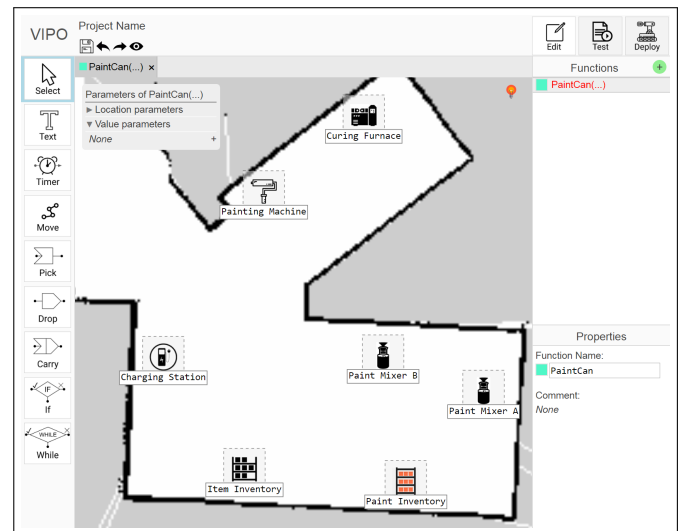
Figure 10. The Vipo IDE displays a toolbar (left), three modes (top-right), and a 2D layout map with IoT machines at the corresponding location (center).
