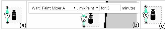
Figure 3. Example of in-place construct: mix paint for 5 minutes. (a) start to create a timer, (b) use popover to select a machine capability and enter required parameters, (c) show estimated time in timer.
