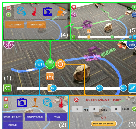
Figure 8: User can insert (1) non-robotic IoT function (2), Time Node (3), or Logic Node with an alternative task line (5) triggered by working status of the connected devices (4).
