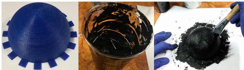
Fig. 18. Fabrication via painting is possible using PDMS and a carbon elastomer mixture which can support 3D objects.
