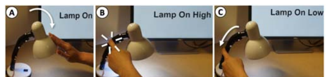
Figure 19. By attaching iSoft , we bring interactivity to a lamp arm.
