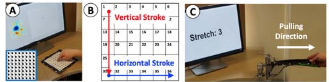
Figure 15. The overall study setup for (A) discrete contact, (B) stroke tracing (i.e., 15x15 cm sensor) and (C) stretching control tasks.
