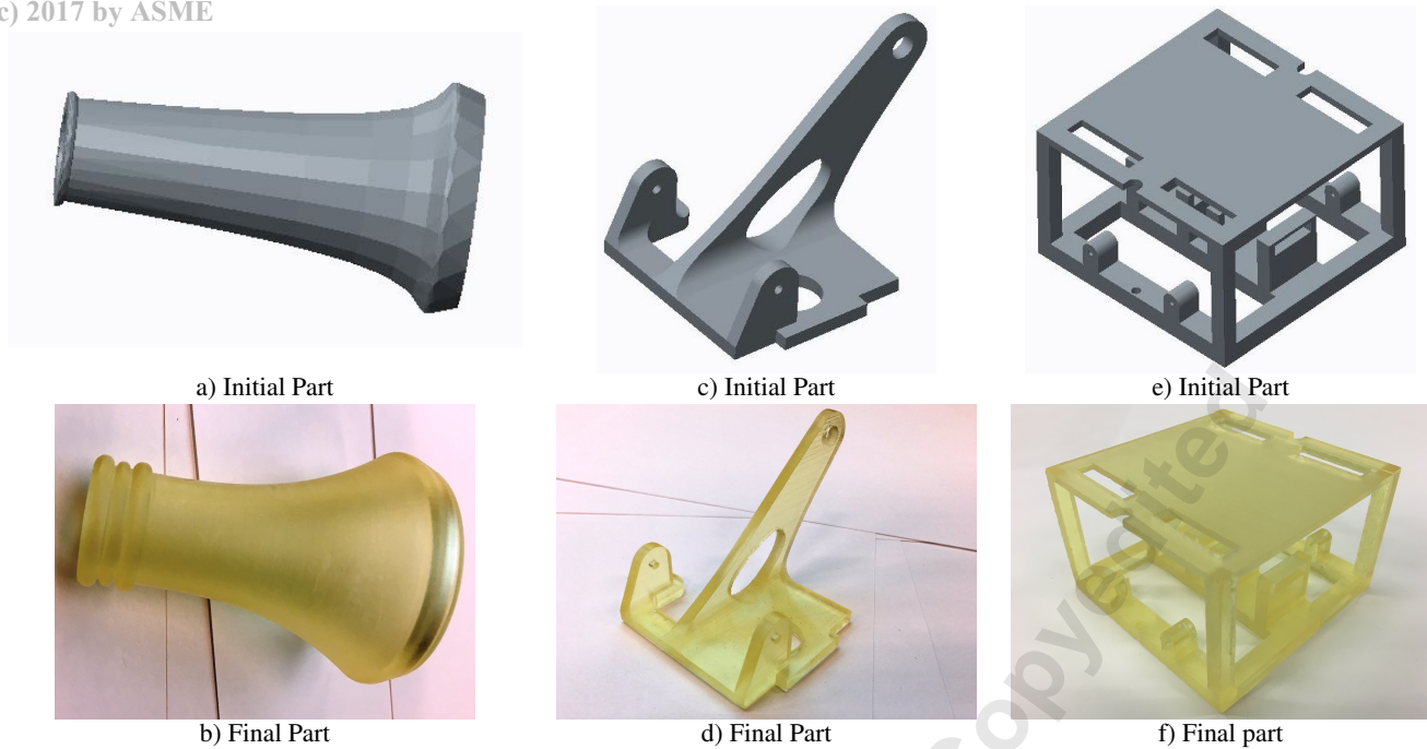
Fig. 3. Examples of parts from the second study. Sub-figures a) and b) show one of only three examples of any changes made. The other two examples show no change from pre to post. All three changes we observed were unrelated to improving the manufacturability.
