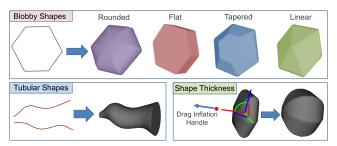
Figure 3. (top) Generating four types of blobby shapes from a profile curve; (bottom left) Generating a tubular shape from two rail curves; (bottom right) Increasing thickness or inflation magnitude of a blobby shape using the 3D manipulation widget.
