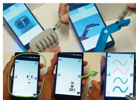
TMotion enables real-time 3D position tracking with an existing mobile device. It supports both discrete and continuous interactions in expanded interaction volume.
