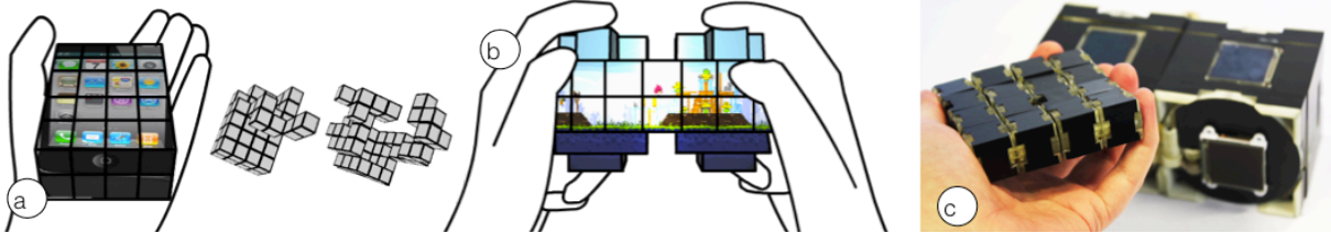
Figure 1. Cubimorph is an interactive device made of a chain of reconfigurable modules that shape-shifts into any shape that can be made out of a chain of cubes, e.g. transforming from (a) a mobile phone to (b) a game console. Following our design rationale, we propose a mechanical design, (c) proof-of concept prototypes and an adaptation of the probabilistic roadmap algorithm for the reconfiguration.
