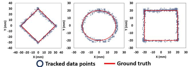
Figure 6. Visualization of the shape tracing at 50mm above the device.
