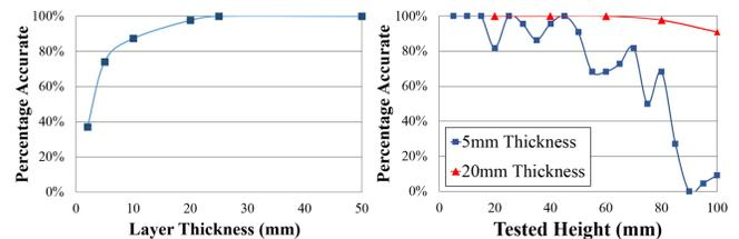
Figure 8. Left: Targeting accuracy with different layer thickness. Right: Targeting accuracy of 20mm and 5mm layer thickness at different heights above the mobile device
