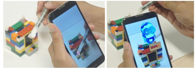
Figure 11. TMotion is aligned with virtual model in the augmented scene (Left). The system enables manipulating virtual blocks with respect to the physical object (Right).
