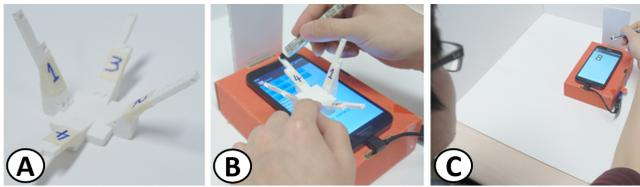
Figure 7. Evaluation task setup: (a) given physical object for measurement, (b) participant measures length of the object (Task 1) and (c) Participant navigates along z-axis for targeting task (Task 2).
