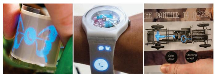
Figure 4. Some examples of deformable touch-sensitive displays fabricated with PrintScreen [6].
