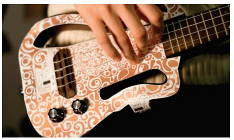
Figure 2. Printed circuits can be both functional and aesthetic. This is a capacitive sensor for music control on an electric ukulele, adapted from an artwork by Evgeny Kiselev. (Courtesy of Nan-Wei Gong)
