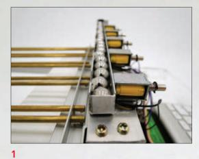
Electronic messages are encoded and transmitted mechanically via steel balls.
