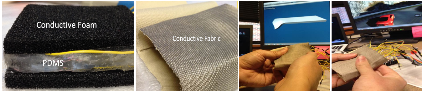
Figure 1: BendID: (a) Layer configuration, (b) Finished Prototype, (c) Localized shape bending, (d) Game controller
