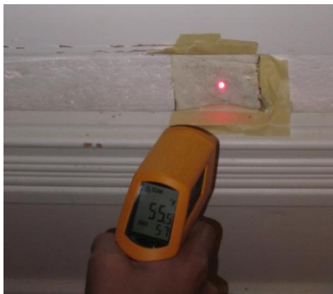
Figure 1: Infra-red measurement gun is shown here recording temperatures during student’s experiment.
