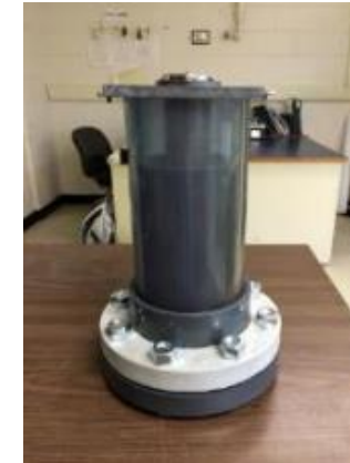
3 L EC unit with biogas pumping
