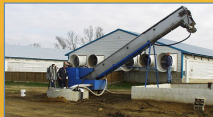
Conveyor screen and a small screw press treating swine manure (Credit: Clemson University Extension)
