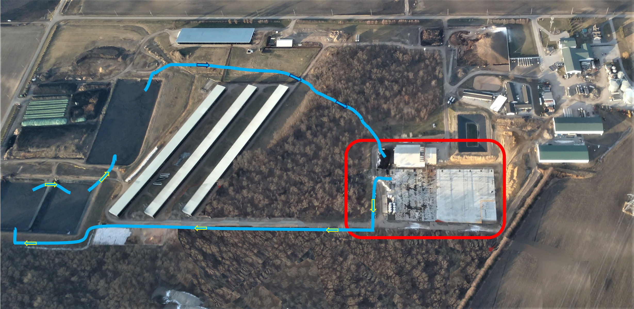
Picture representation of make-up water loop on farm
