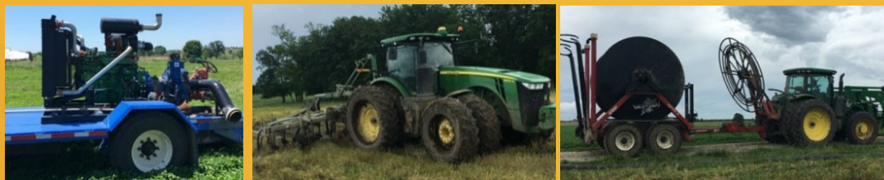
Booster pump (left), application toolbar/tractor (center), and hose cart/humper (right).
