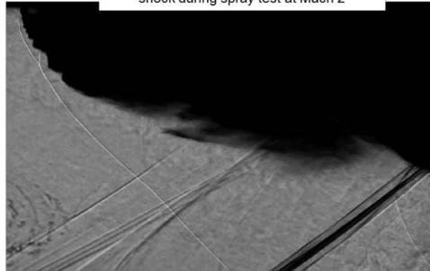
Research is underway at a more fundamental level at Mach 2 to characterize sprays in a fully optical accessible test section. The liquid jet is monitored using multiple techniques such as kHz shadowgraphy, backlit imaging, and Mie Scattering. This figure shows some experiments performed in the Linear Experimental Aerothermal Facility (LEAF).
