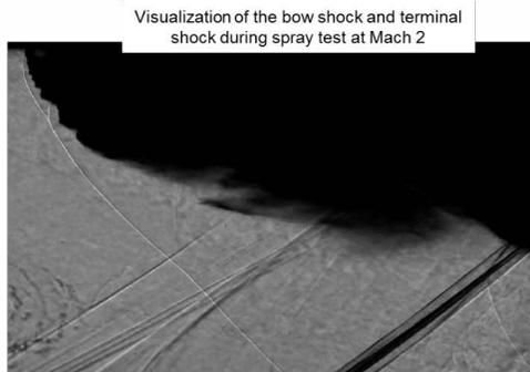
Research is underway at a more fundamental level at Mach 2 to characterize sprays in a fully optical accessible test section. The liquid jet is monitored using multiple techniques such as kHz shadowgraphy, backlit imaging, and Mie Scattering. This figure shows some experiments performed in the Linear Experimental Aerothermal Facility (LEAF).
