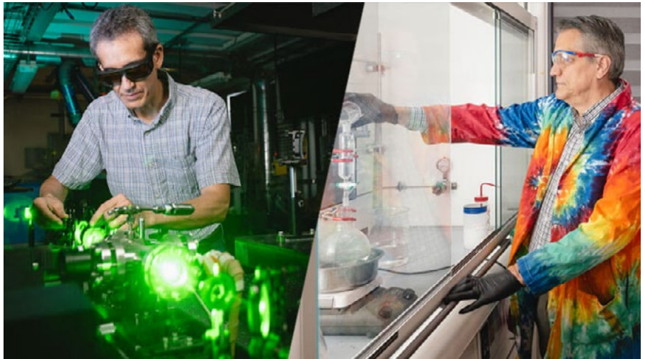
(Left) Terrence Meyer, professor of mechanical engineering, uses laser diagnostics to measure solid fuels' gas compositions after burning. (Right) Steven Son, the Alfred J. McAllister Professor of Mechanical Engineering, prepares a mixture for the synthesis of a solid fuel used in a rotating detonation engine (RDE).
