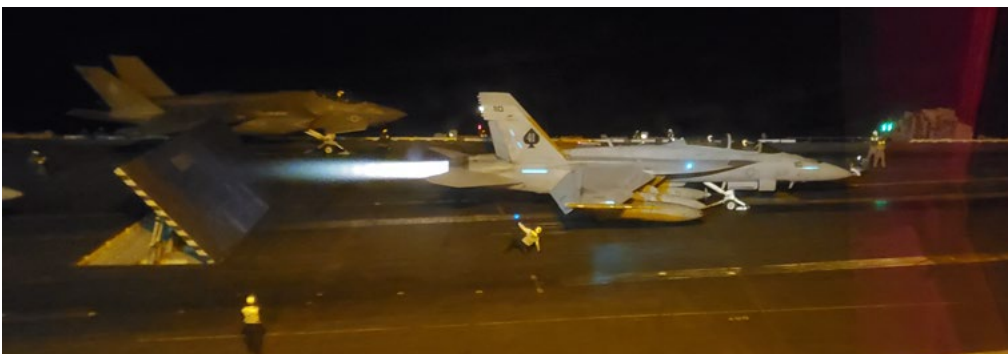
An F-18 operated by the U.S. Navy fires up its afterburners in preparation for a heavy catapult launch on the flight deck of the USS Abraham Lincoln.
