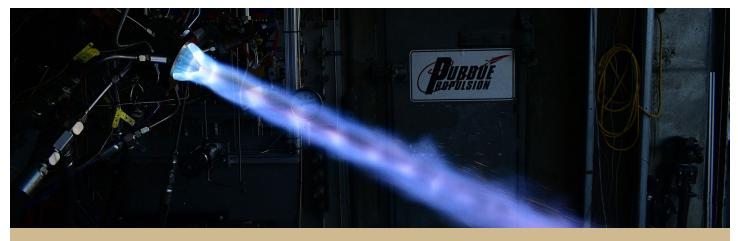
Purdue researchers are leading in study and design of 3D-printed rotating detonation rocket engines, which could transform spacecraft and hypersonic vehicles. (Purdue University photo/Ariana Martinez)
