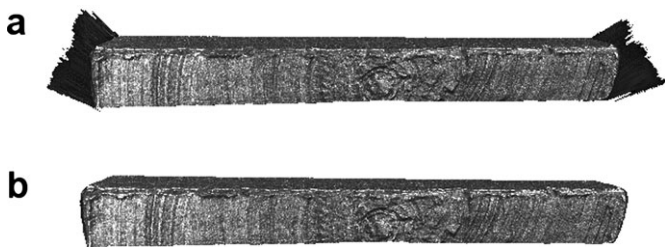
FIG. 5—Tip 8 Side A with overlaid 2D texture. (a) Before cleaning. (b) After cleaning.
