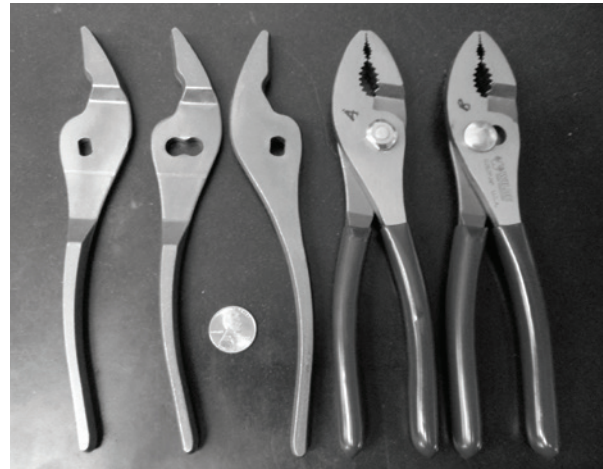
Figure 1: Slip-joint pliers in their unfinished and finished states. From left to right: plier halves (single and double hole) before broaching; an example flat side of pliers that will be polished; finished and labeled pliers (sides A and B).
