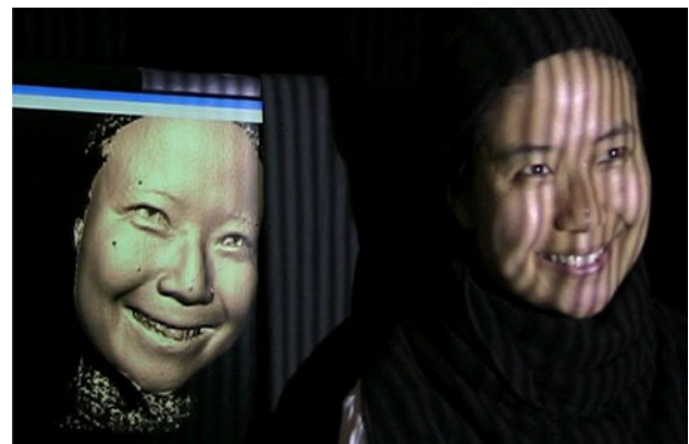
Fig. 11 Simultaneous 3D data acquisition, reconstruction, and display. The system achieved a real-time 3D imaging at a frame rate of 30 fps with an image resolution of 640 \times 480 per frame
