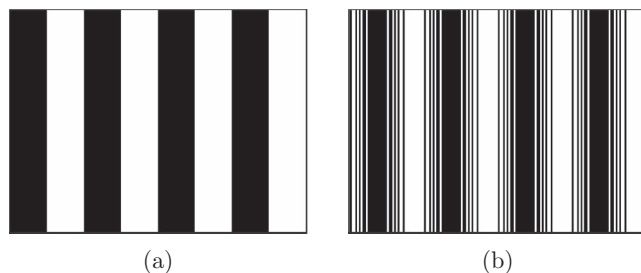
Fig. 3 Comparison of computer-generated binary patterns: (a) One of the SBM patterns and (b) one of the OPWM patterns.
