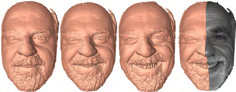
Fig. 11. Measurement result of human facial expressions. The data is acquired at 60 Hz, the camera resolution is 640 \times 480 .
